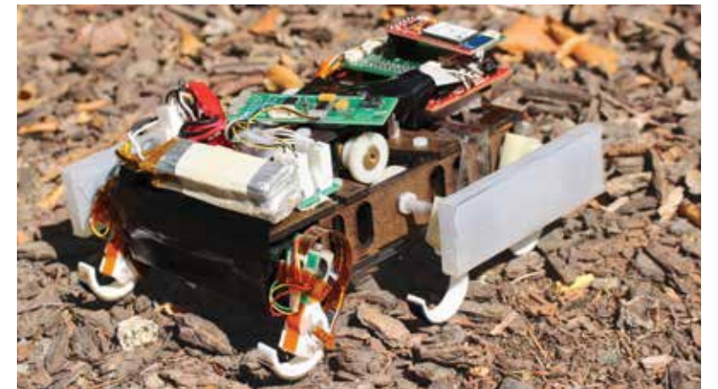
A small running robot named SAIL-R (top) has tactile sensors attached to six C-shaped legs (left). When the legs whirl around and smack the ground, the sensors detect the impact forces, which could help the machine choose an appropriate walking gait.
