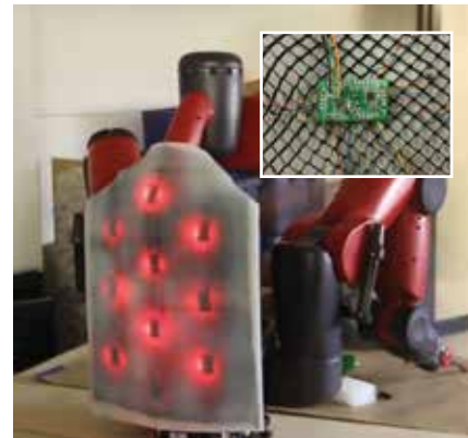
A rubbery, artificial skin covers the back of a robot named Baxter. The skin contains 10 sensor nodes — vibration sensors coupled with tiny computers (inset) that let the skin detect different textures.
