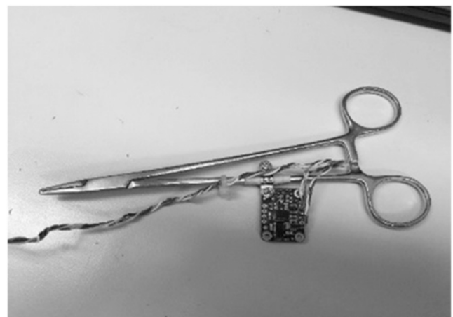
FIG. 3. Ardafruit BN0055 nine-degree-of-freedom sensor attached to needle driver.
