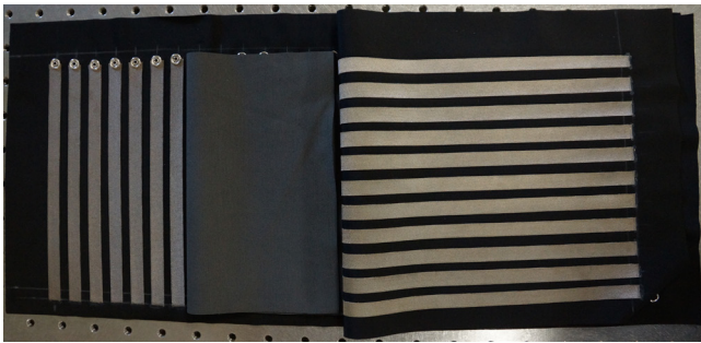
Figure 3. Sensor construction with columns and rows of conductive fabric. The gray resistive material is folded back to reveal columns of conductive material. Metal snaps are located at the top of each column.
